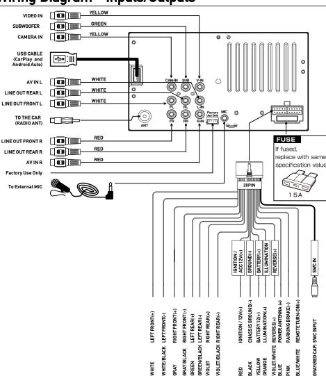
When replacing a fuse, make sure to use the correct type and amperage. Using an incorrect fuse could cause damage. The unit uses (1) 15 amp ATC mini style fuse located on the power connector
