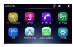
In main menu, press the desired icon to enter the corresponding mode: FM Transmitter/Device/BT Phone/BT Music/USB/Android/Apple/Settings.
