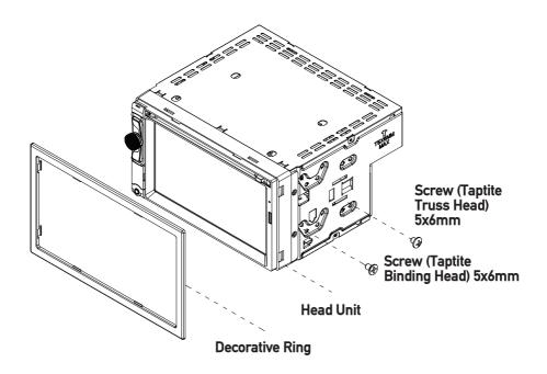
TYPICAL FRONT-LOAD MOUNTING METHOD
